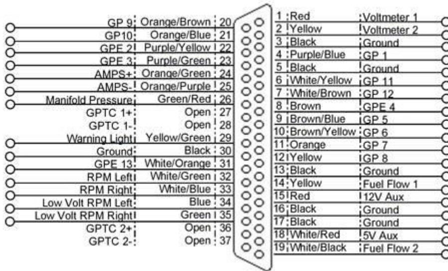
Figure 26– SV-EMS-220 37-pin Main Sensor Harness Female D37 Pin Insertion View (Rear)
