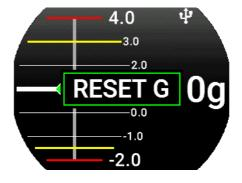
Push the knob again to reset or wait 5 seconds to go back to the main screen without reset.
