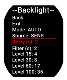
**Delay (s):** It introduces a delay to the variation of the backlight, it can be useful to avoid continuous changes in brightness when the sensor is hit by light and shadow alternately.
