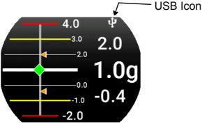
To activate the Logger choose "Yes" from the Main Menu>Logger. The icon will turn **green** when the file is being written and **red** when the Logger is enabled but the USB stick is not connected.
