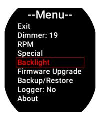
**Exit:** confirm to "exit" from the setup menu and go back to the main screen.
