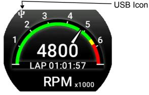
To activate the Logger choose "Yes" from the Main Menu>Logger. The icon will turn **green** when the file is being written and **red** when the Logger is enabled but the USB stick is not connected.
