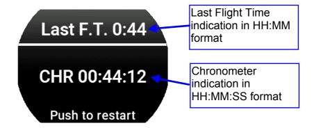
Push the knob to restart the Chronometer. This feature is useful to restart the chronometer with a simple click when you arrive at the waypoint. The Chronometer screen automatically disappears if you don't press or rotate the knob for 5 seconds. As soon as you press it, you return to the main screen.
