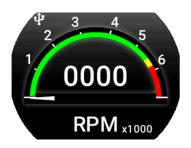
Full scale 7000 RPM for Rotax 912, Rotax, 914, Rotax 912iS, Rotax 915iS engines.
