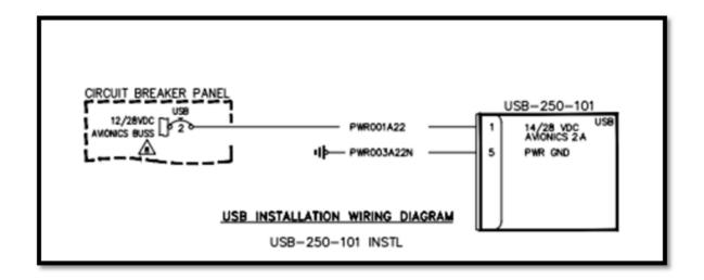
(f) If a jumper wire is required to connect the USB charger to the CB, use 20 Guage MIL-W-22759/16 or equivalent wire. Wiring is to be performed in accordance with AC 43.13-1B, 2A, acceptable methods, techniques and practices. These instructions are available online here.
