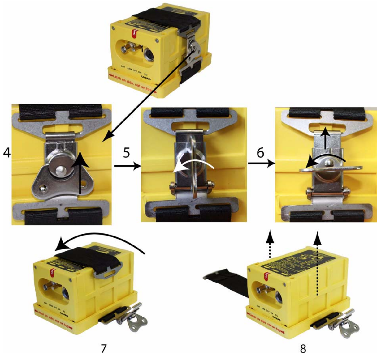
Figure 207: ELT removal from a draw latch mounting bracket
